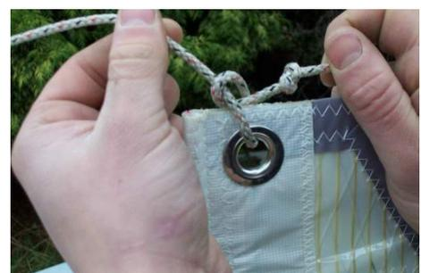
Pull the rope tight so that the rope binds on the original overhand knot.
