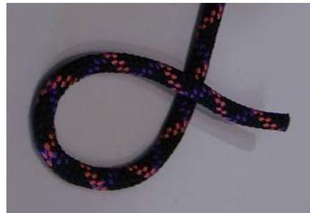
Lead the tail underneath the standing end of the rope
